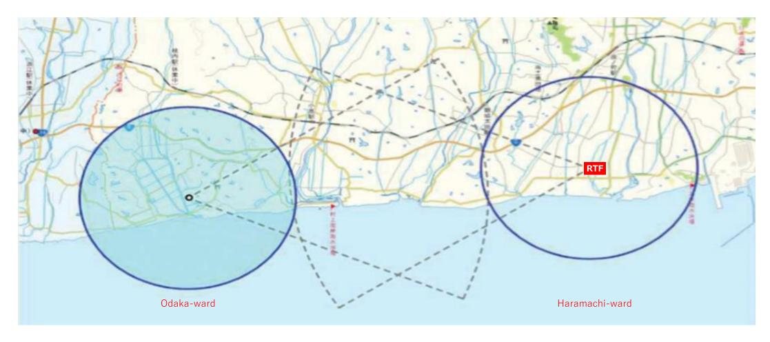
Two communication towers in Haramachi (In the RTF) and Odaka ward. Each communication tower has four antennas that 2.4GHz/920MHz rod antennas (2 km in radius) and 2.4GHz/920MHz directional antennas (8 km in radius). Competitors always activate only one of the four antennas and fly long distances.
